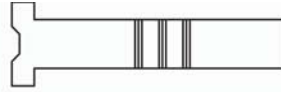
Tailpiece for Maxum® Deadbolt Lock, outside cylinder, 1.430" length for doors over 1 3/4" thick CT-Y61
